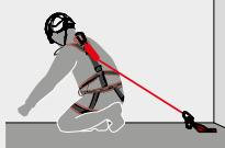
Where the risk of falls cannot be eliminated, use a suitable safety system to minimise the consequences, employing restraint or fall protection systems.
