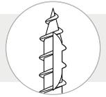
viti inserite **SENZA** preforo  $\rho_k \leq 420 \text{ kg/m}^3$
