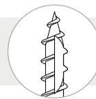
viti inserite **SENZA** preforo  $\rho_k \leq 420 \text{ kg/m}^3$
