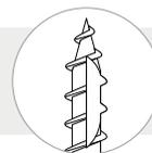
viti inserite **SENZA** preforo  $\rho_k \leq 420 \text{ kg/m}^3$
