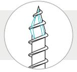
viti inserite **SENZA** preforo  $\rho_k \leq 420 \text{ kg/m}^3$
