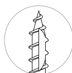
standard tip SHARP 1 CUT type RBN / RBN2
